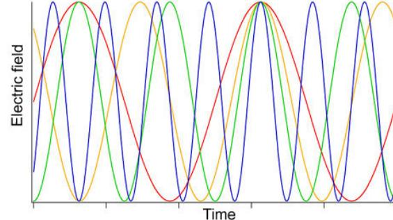
A titanium-sapphire laser has a gain bandwidth of approximately 100 THz centered at 800 nm.
